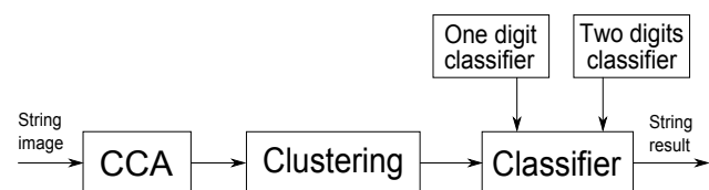
Figure 1. Numeral string recognition system (CCA = connected component analyzer).
