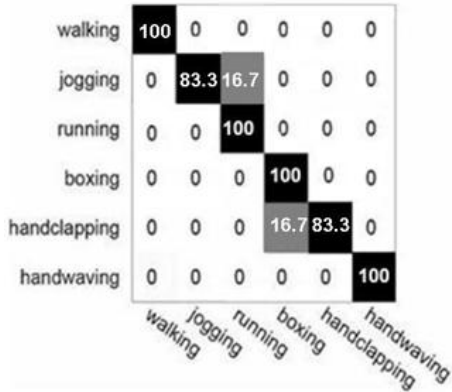
Fig. 7: Confusion matrix achieved by our Unsupervised classification algorithm with MMD on KTH human action dataset. The overall accuracy rate of 94.4% is achieved with this method.
