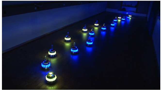
Fig. 12. Foot-bots moving in a dynamic chain between two targets
